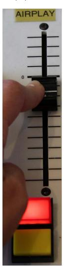
The needles on the sound level meters will start to bounce – adjust the fader level so that the needles rarely bounce into the red area.
